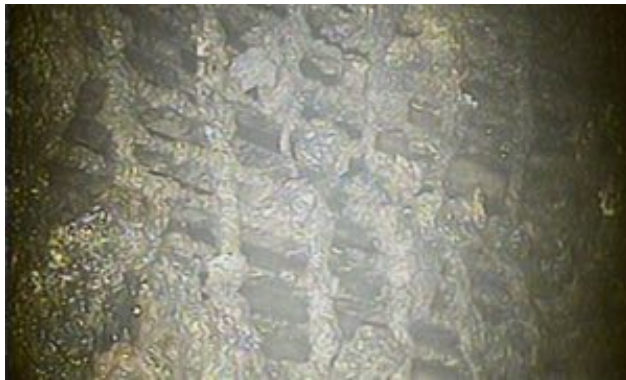
Material found below the damaged No 2 reactor at Fukushima nuclear plant, believed to be melted fuel, from footage taken on 30 January. Photograph: Reuters
