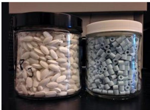
**Powerful pills:** Two versions of catalysts developed by Siluria to convert natural gas into ethylene, which can be used to make gasoline and chemicals.
