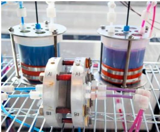
**Liquid energy:** Novel energy storage materials flow from the white containers shown here into a fuel-cell like device in the foreground, where they generate electricity.
