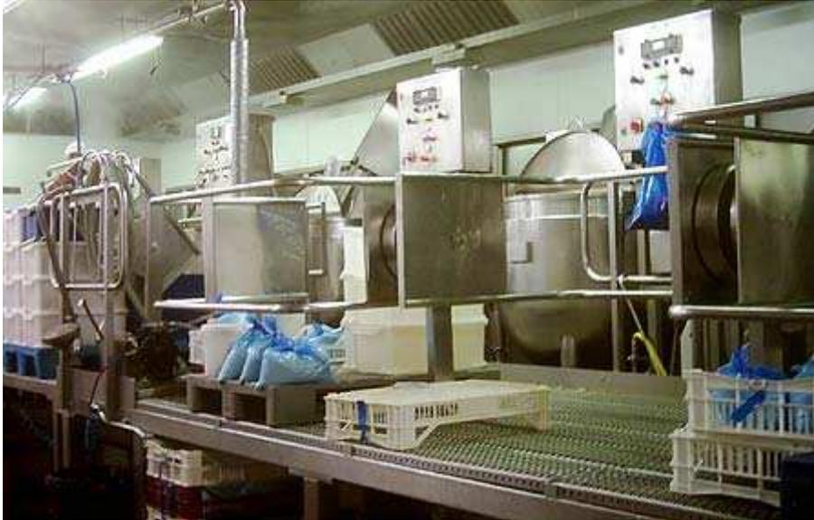
Image: The cook pans where the various foods are cooked. Computer systems monitor the time, temperature and status of the products. The chefs working here are all experienced in the catering trade.
