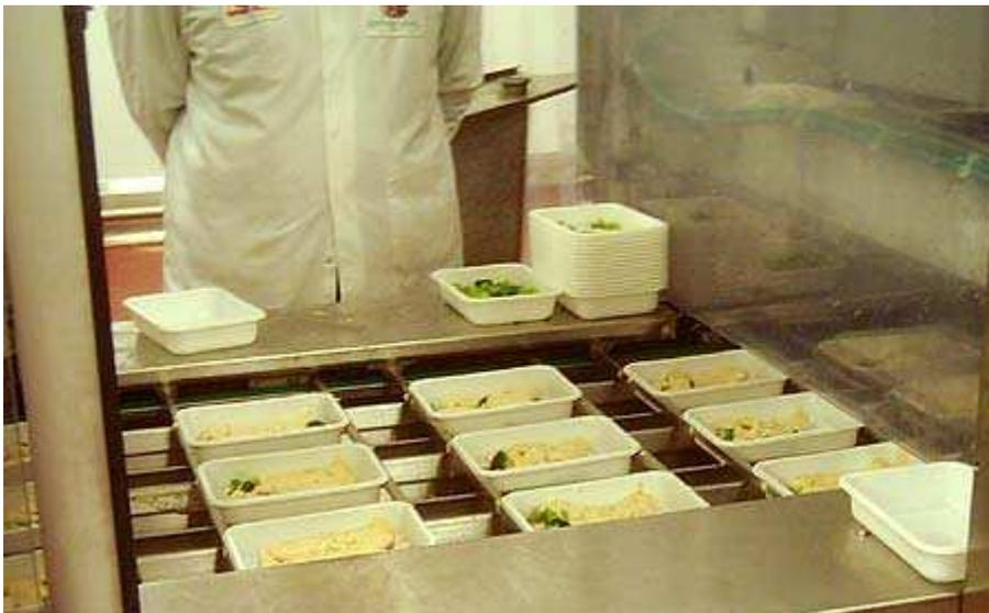
Image: Chicken and Broccoli Pies pass through the watchful eyes of a quality checker before having the potato topping added by machine. The staff member can add additional pieces of broccoli by hand if they spot that more is needed.
